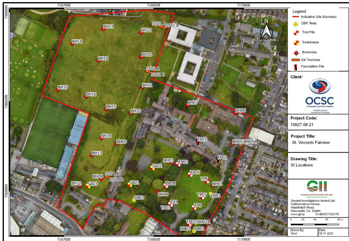
Figure 5.4 Site Investigation Points (Source: GII, Ground Investigation Report, 2022). Note: Site Boundary is associated to site investigation only.
