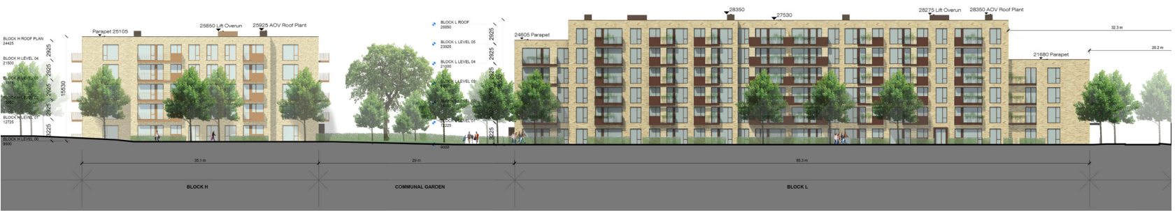
Excerpt from SVRD-STW-ST-ZZ-DR-A-024002 - Convent Quarter and Garden Quarter - South Elevations of Buildings H and L showing staggered parapet
