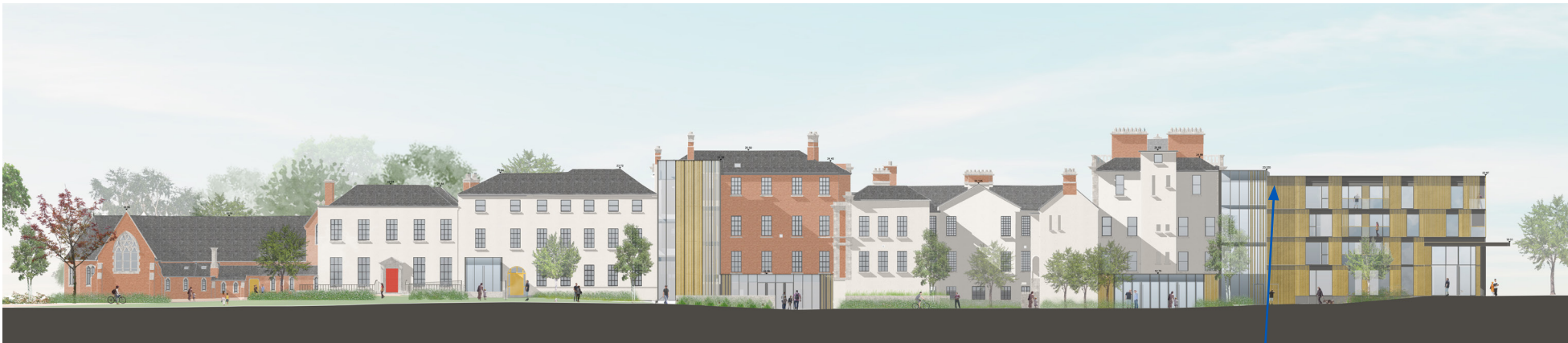
Building K - Protected/historic Structure and Building J - North Elevation - showing Building J set below the eaves/parapet of the Protected Structure
