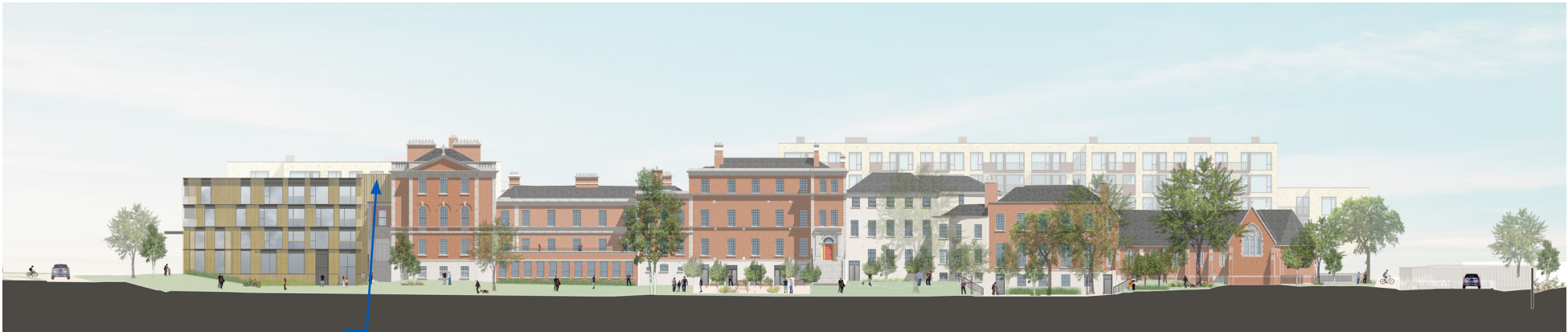
Building K - Protected/historic Structure and Building J - North Elevation - showing Building J set below the eaves/parapet of the Protected Structure
