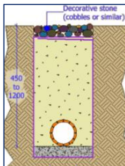
Figure 3.6 - Filter Drain under pavement (left)
