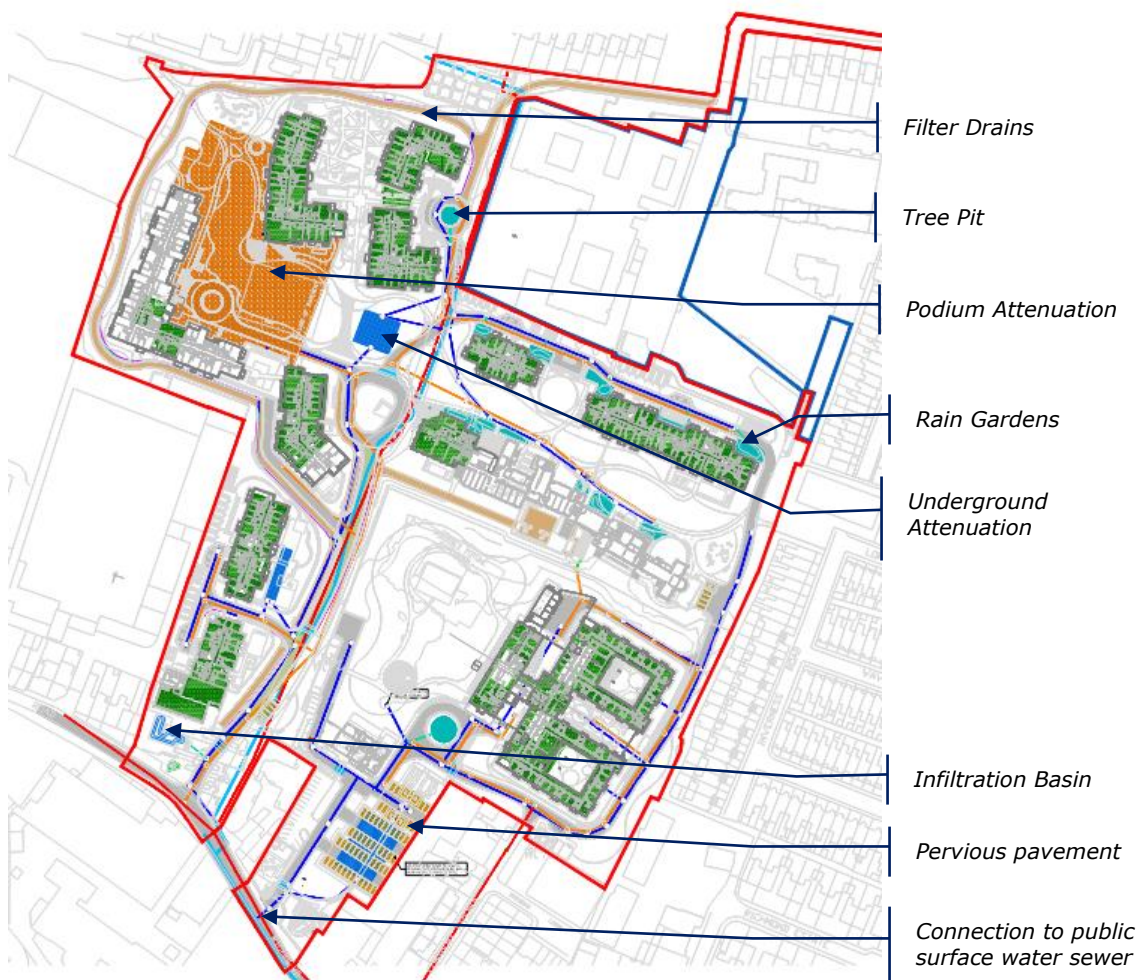
Figure 3.4 - Proposed Surface Water Drainage Strategy
