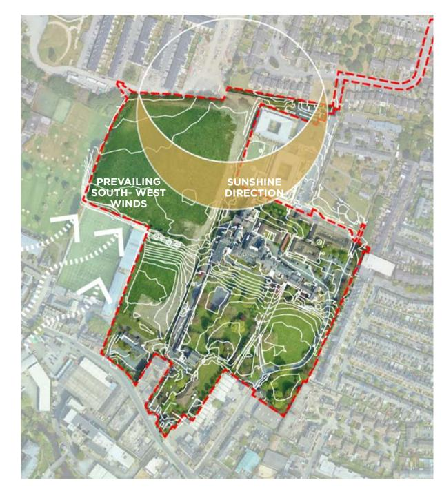
The site is divided, topographically, into two portions by a singular embankment level change of approximately 4-5m, running east west and centrally traversing the site.
